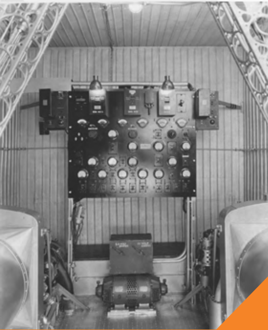
Generator room and instrument panel of the USS Akron airship. Photo from the Frederick J. Ilse Collection.
